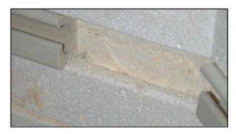
Using Linemen's Pliers snap off the BOTTOM edge of the holder (note carefully the fact that the BOTTOM of the groove is closest to the edge that you are breaking off.:
