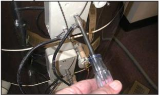
5) Cut the old elements off as close to the "through hole" on the outside of the kiln as possible. You want a straight element tail to pull through the through hole, not a crooked one.
