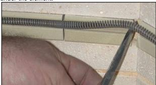
Lift Elements out of the groove of the ceramic holders:
