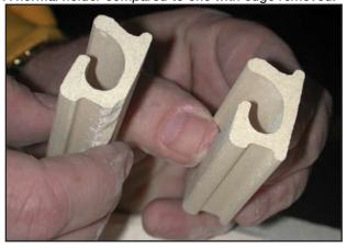
You can now just snap the new holder into the slot in the firebrick. It will hold in place with no cement:
