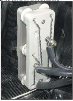
Parallel circuits are another way of wiring elements in the kiln. The element connection bolts in these circuits have two or more element tails wrapped around them; all the bolts have power wires attached to them. Parallel circuits use only two element connection bolts per circuit. The power is applied to the beginning and end of ALL the elements at once. Thus the resistance of the entire circuit is the number of elements in the circuit divided into the factory resistance value for one element.
