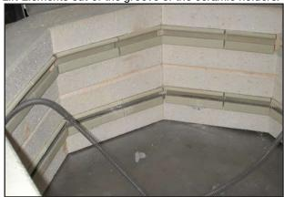
Sometimes very old elements can become wedged in the element holders, making it necessary to carefully pry/twist/ break them out. A propane torch or just turning the kiln on for a few minutes (if it will come on) will soften the wire of the elements and make them easier to get out. Use heat protecting gloves such as welding gloves or heat treating gloves (you can buy these from L&L) and a pair of needle nose
