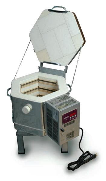
The Doll/Test kilns are meant for small ceramic work such as dolls, for testing glazes without firing a large load, and for other laboratory and home uses. It is available with two different controls and in 15 amp (Cone 5) or 18 amp (Cone 10) 120 volt versions or various high voltage versions for extra power and higher temperatures.
