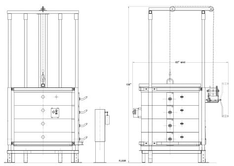
The kiln shown at the top is the X3236-D. The one below is the T3445-D. All the 45" high models have the height of this T3445-D. All the 36", 27" and 18" high models have the height of the X3236-D.
