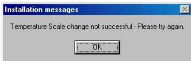
This message box is displayed if the message sent from KISS to the controller to change the temperature scale does not complete successfully. The message may not have been transmitted correctly or the data received from the controller during the verification process may have contained noise.
