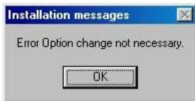
This error message is displayed when the user has selected to either turn on the error checking feature when it's already on or when the user has selected to turn off the error checking feature when it's already off. It is an informational message to let the user know that KISS has not sent a new message to the controller about the error checking.
