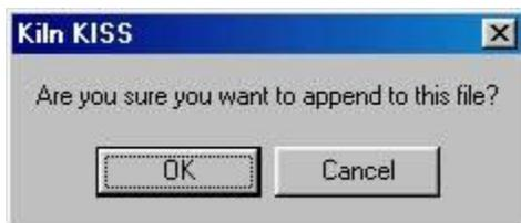
By selecting the “OK” command button, the user will be adding firing information to the end of the current file on the disk and, by selecting the “Cancel” command button, the user will be able to enter a different filename for this firing’s data.
