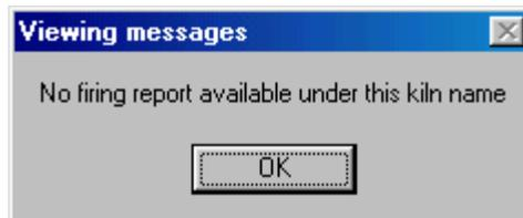
1. The controller must be set up to be creating a firing report in the Menu Screen. If that option button has not been set to “Yes”, the firing reports will not be created.
